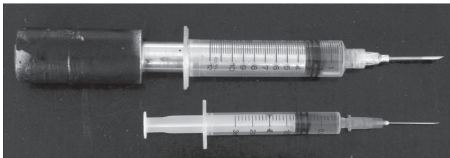
Fig. 1. The 10-mL Paxarms pole syringe (upper), consisting of a metal base (55 mm long), a metal plunger (75 mm long) with a black rubber piston and a 1.6 \times 25 -mm needle, compared with a standard 3-mL syringe (lower) loaded with a 0.8 \times 25 -mm needle.
